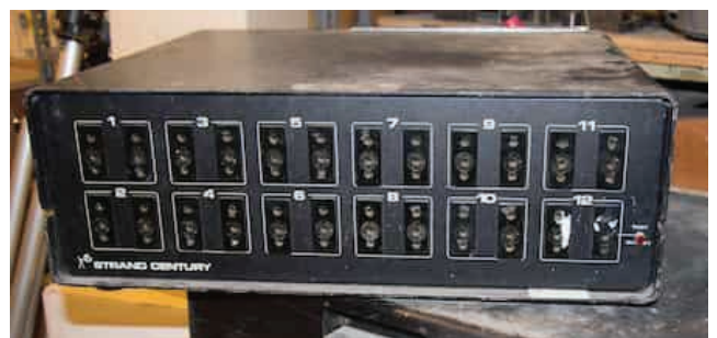
Below: a CD-80 2.4k dimmer pack. Popular for touring - with (12) dimmers in a single module.
